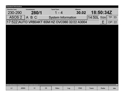
VIDS uses redundant file servers with hubs, workstations, video integration components, audio components, 100BaseT Ethernet, and fiber optics to interface and manage all the system data. The network operating system is Windows NT 4.0. The display software was developed to support the requirements of each system interfacing with VIDS to maximize the information available to the user.
